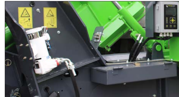
Dust suppression pump
