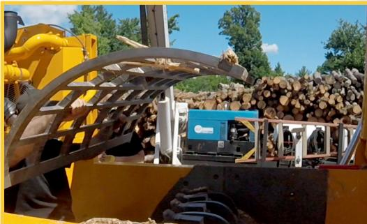
60" wide cleated discharge belt provides unrestricted discharge of ground product.
