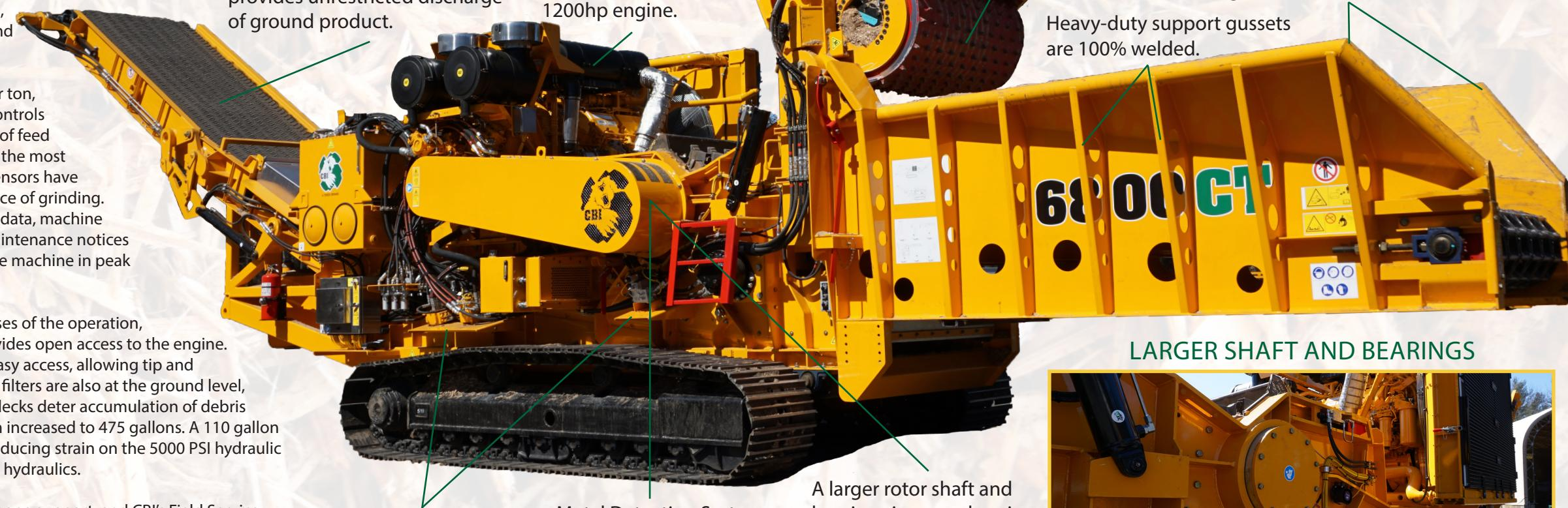
Split hog box for ease of maintenance. The entire grinding chamber rises for quick tip and screen changes.
