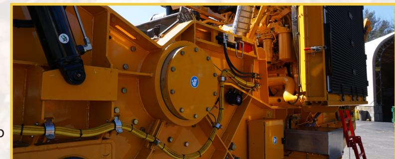
A larger rotor shaft and bearings increase bearing life and allow for a 1200hp CAT C32 engine.
